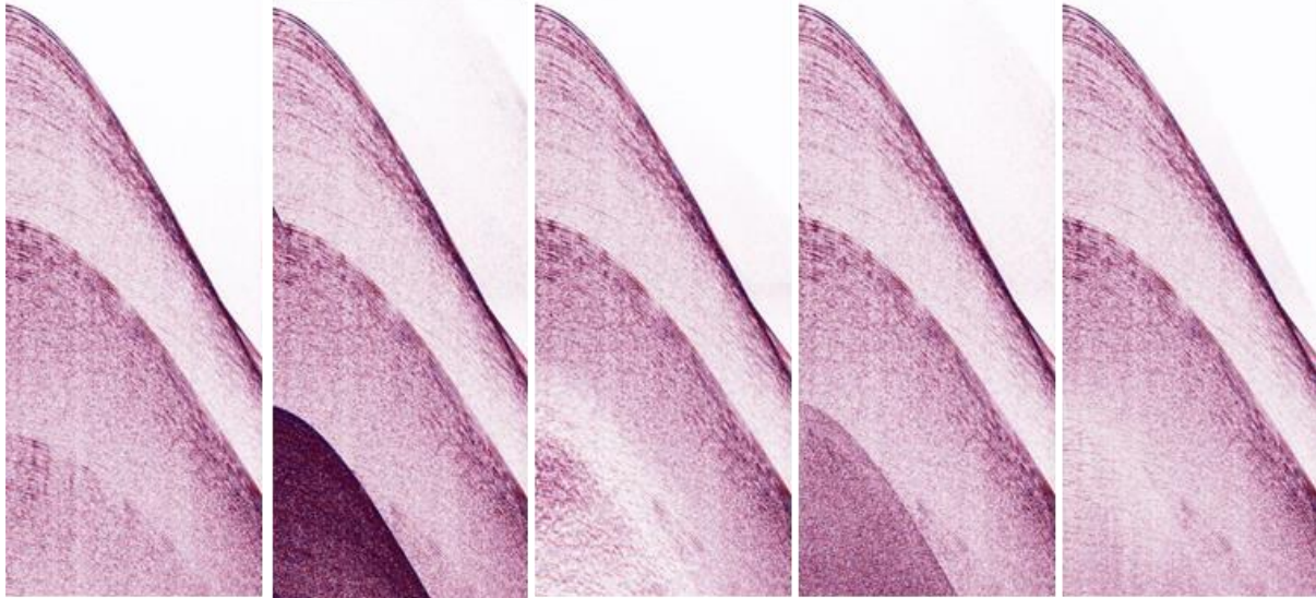
Figure 3: Impact of different deblending techniques. From Left to Right: Unblended data, Data with interfering shot, 3 examples of separated results showing obvious differences
